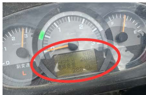
On the combine's operator monitor, you can view: "Average protein content", "Moisture content", "Cumulative weight"
