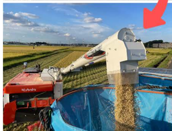
The combine harvester used for harvesting. The harvested and threshed rice grains are transferred into flexible container bags for transportation.
